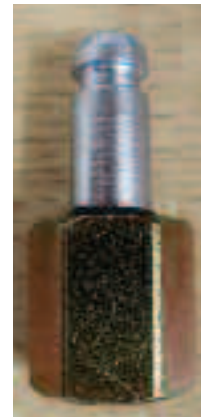
ASNU 121 INJECTOR TO FUEL RAIL COUPLING FOR SIEMENS PIEZO INJECTORS
