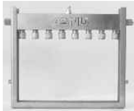
ASNU 122 FUEL RAIL FOR SIEMANS PIEZO INJECTORS
